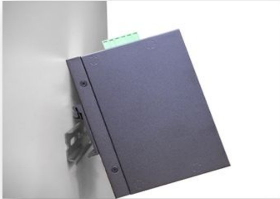
Figure 3.2 - Insert the Switch on the DIN-Rail
