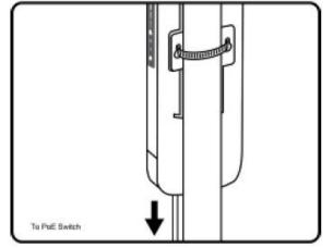
Figure 3.1 - Example of Mounting the Device on the Pole
