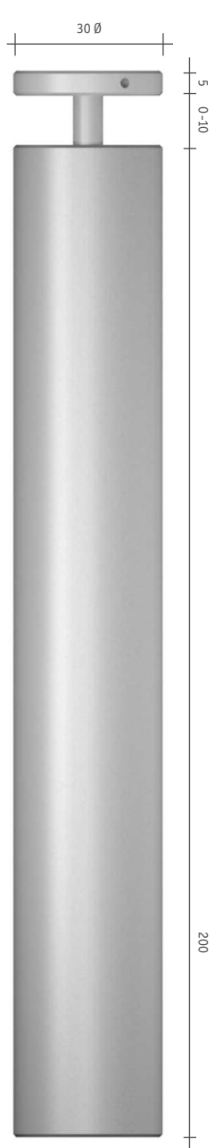
PSD.5 Panel support for drilled sheet
