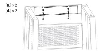
**STEP 11** Use eight (8) M6x14 screws [**a**.] to attach two (2) wheel assemblies and one (1) cart side panel to one (1) cart frame. Repeat with the other cart frame.
