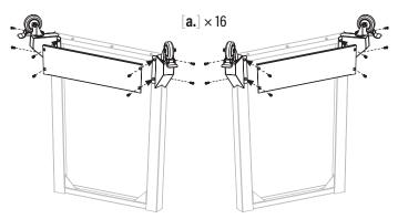
**<u>STEP 13</u>** Use four (4) M6x14 screws [a.] to attach the front cart panel to the cart frames.
