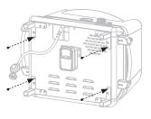
**<u>STEP 03</u>** Slide the four (4) feet onto the legs.
