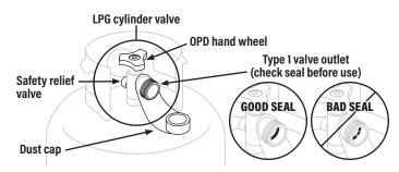
The seal on the type 1 valve outlet could, over time, show marked and visible damage or deterioration that might cause a leak even with the connection tightened.
