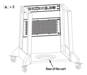
**STEP 15** Use four (4) M6x14 screws [**a**.] to attach the rear cart panel to the cart frames. (Be sure that the angles match. DO NOT install upside down.)
