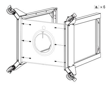
**<u>STEP 14</u>** Use two (2) M6x14 screws [**a**.] and two (2) M6 nuts [**d**.] to attach the orange background panel to the front logo panel. **Note:** D0 N0T fully tighten screws yet.
