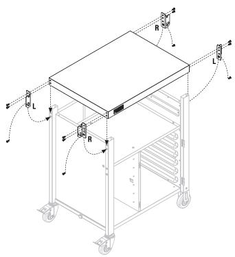
STEP 10 Use four (4) M6x15 bolts to attach the left garbage bag holder bracket and the logo panel to the cart assembly.
