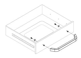
**STEP 12** Pull out the two (2) drawer sliding tracks from the side panels. Insert the drawer rails into the cart tracks.
