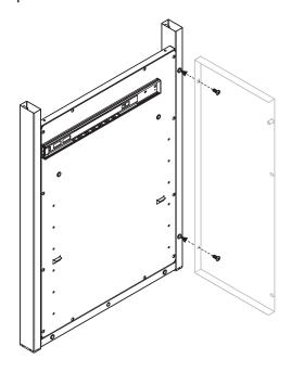
STEP 03 Use two (2) thumb screws to attach the cart base to the left and right side panels.
