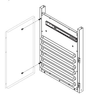
STEP 04 Use four (4) M6x15 bolts to secure the cart base to the left and right side panels.
