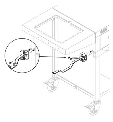
**STEP 19** Use four (4) wing screws, four (4) washers and four (4) slotted washers to attach four (4) shelf hooks into the left side shelf. Repeat with the right side shelf.
