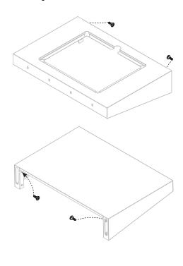
STEP 17 Hang the upper step bolts on the side shelf brackets. Use two (2) M6x12 step bolts to secure the left side shelf to the brackets. Repeat with the right side shelf.
