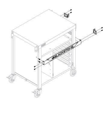
STEP 11 Use two (2) M6x15 bolts and two (2) washers to attach one (1) handle to the drawer face.
