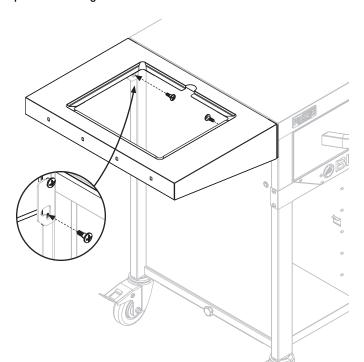
$\underline{\text{STEP 18}}$  Use two (2) M6x15 bolts to attach the paper towel holder to the left side panel.
