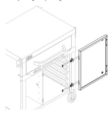
**STEP 15** Use four (4) M4x10 step bolts to attach the garbage bag holder to the garbage bag holder brackets.
