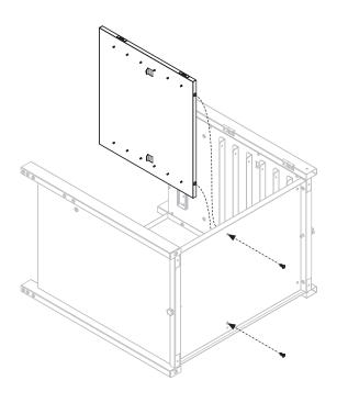
$\underline{\textbf{STEP 06}}$  Use four (4) M6x15 bolts to attach the horizontal partition to the left and right side panels.
