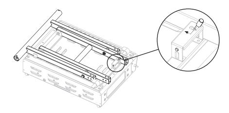
**STEP 02** Use twelve (12) M6x12 bolts to install the upper legs onto the wheeled leg assembly.
