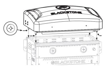
**STEP 07** Use two (2) M6x20 screws (**a**) to attach the hood handle, two (2) hood handle bezels (**j**), and stopper bracket to the griddle hood.
