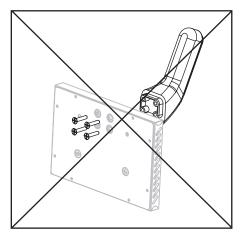
Be sure to install handle correctly, with the handle facing down.
