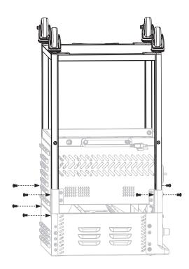
**STEP 04** Use four (4) thumbscrews (**k**) to secure the legs to the airfryer body.
