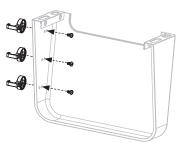
**STEP 14** Thread two (2) M6 step bolts (**c**) into the top holes of the left side shelf. Repeat with the right side shelf.
