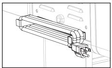
Wrap the power cord around the power cord bracket when the air fryer is not in use.
