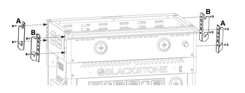
**STEP 05** With the help of another person, place the griddle unit on its wheels. Use eight (8) M6x15 screws (i) to attach the four (4) side shelf brackets
