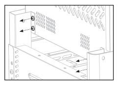
Before proceeding, loosen all eight (8) screws on the left and right sides of the griddle body assembly one (1) turn.
