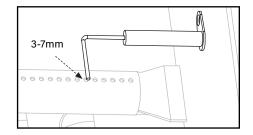
Ensure that the ignition needle is positioned 3-7mm away from the burner tube, positioned above a burner hole.
