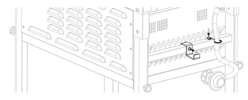
**STEP 12** Use two (2) M6x12 screws (**g**) to attach the power cord bracket to the right side of the griddle.
