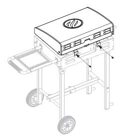
**STEP 12** Use the two M6x16 screws pre-installed in the hood handle to attach the hood handle and two (2) hood handle grommets to the hood.
