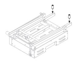
**STEP 02 1** Pull the locking pin to unlock the right leg assembly.
