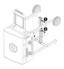
**STEP 03 1** Pull the far ring pin to lock the crossbar. **2** Pull the inner left ring pin to fold the left leg assembly.
