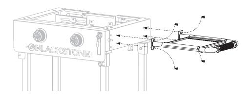
**STEP 09** Use the two (2) M6x12 bolts pre-installed in the side handle to attach the side handle to the left side of the griddle.
