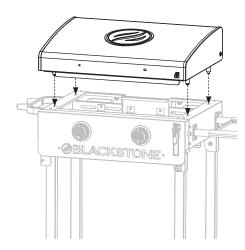
**STEP 11** Use two (2) M6x12 bolts to secure the back of the griddle top and hood to the back of the griddle body.
