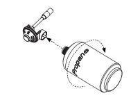
**STEP 15** Insert the gas regulator into the fuel line of the griddle. Turn the collar of the gas regulator clockwise to secure it to the fuel line.
