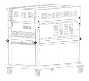
**STEP 11** Unscrew the two (2) M6x12 screws from the right side of the griddle, then use these screws to attach the power cord bracket to the right side of the griddle.
