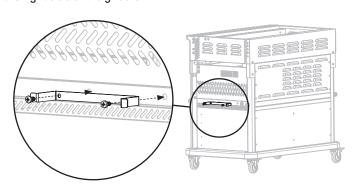
$\underline{\textbf{STEP 12}}$  Use two (2) M5x10 screws [b.] to attach the paper towel holder to the right-front leg.
