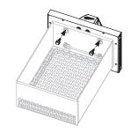
**STEP 27** Place the cutting board onto the right side shelf.
