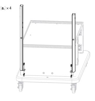
**STEP 07** Use four (4) M6x12 screws [a.] to attach the right-front leg and right-rear leg to the cart base. (Note: the front leg is shorter than the rear leg.)
