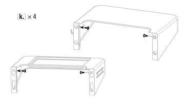
**STEP 25** Slide the left side shelf onto the side shelf brackets. The threaded M6 step bolts will hook and hold the shelf.
