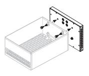
② Use four (4) M5x15 screws [j.] to attach the drawer handle to the front panel. Be sure to install handle correctly, with the handle facing down.
