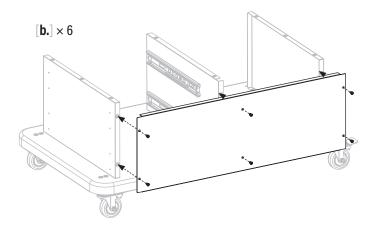
**STEP 05** Use eight (8) M5x10 screws [**b**.] to attach the top cart panel to the left cart panel, middle cart panel and right cart panel.
