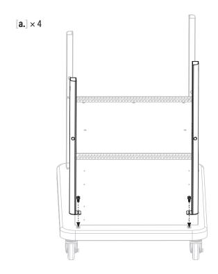
**STEP 08** Use four (4) M5x10 screws [b.] to attach the crossbar assembly to the left-front and left-rear legs.
