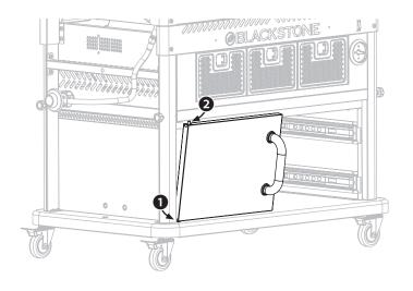
**STEP 15** Use seven (7) M5x10 screws [**b.**] to attach the cart drawer front panel to the cart drawer body. Repeat this step with the other drawer.
