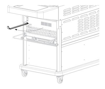
**STEP 32** Hang the rear grease cup with aluminum foil liner on the back of the unit.
