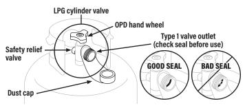
The seal on the type 1 valve outlet could, over time, show marked and visible damage or deterioration that might cause a leak even with the connection tightened.
