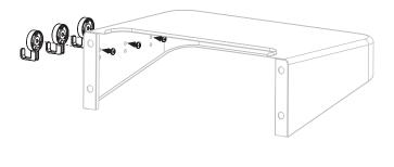
**STEP 24** Thread two (2) short M6 step bolts  $[\mathbf{k}.]$  into the top holes on the left side shelf. Repeat with the right side shelf.
