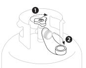
STEP 02 Hold the regulator in a straight line with the Type 1 valve outlet so as not to cross thread the connection.
