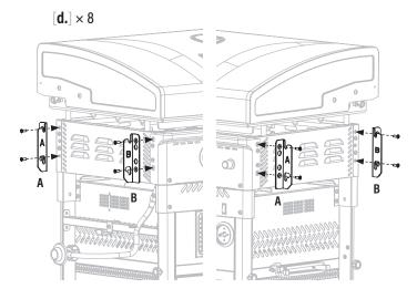
**STEP 23** Unscrew the three (3) M6x8 screws from the side shelf pegs. Use the (3) M6x8 screws to attach the three (3) side shelf pegs to the left side shelf.
