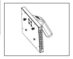
Keep the handle assembly with your Griddle, reassemble after the fryer drawer is clean and dry.
