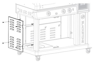
**STEP 13** Use four (4) M4x10 screws to attach two (2) shelf brackets to the right panel.
