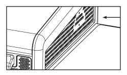
To verify that the air fryer burner has lit, look into the burner chamber from the right side of the unit.
