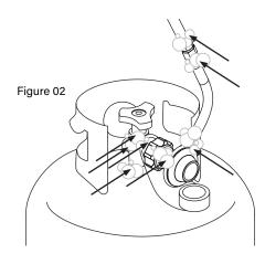
**STEP 03** Immediately close the LPG tank by turning the OPD hand wheel clockwise and re-tighten connections. If leaks cannot be stopped **DO NOT TRY TO REPAIR.**
