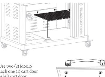
**STEP 16** Use two (2) M6x15 screws to attach one (1) cart door handle to the left cart door.
