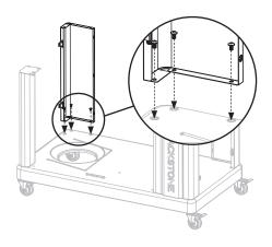
**STEP 07** Use four (4) M4x10 screws to attach two (2) shelf brackets to the back panel.
