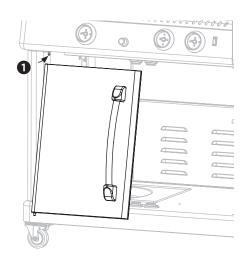
**STEP 18** Use two (2) M6x15 screws to attach one (1) cart door handle to the right cart door.
