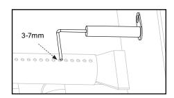
Ensure that the ignition needle is positioned 3-7mm away from the burner tube, positioned above a burner hole.
