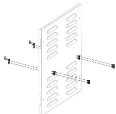
**STEP 14** Use four (4) M5x10 screws to attach the right panel to the right legs.
