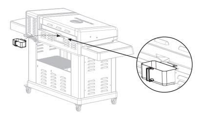
**STEP 26** Install the three (3) control knobs by pushing them into place in the OFF position.
