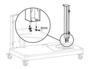
**STEP 05** Use three (3) M6x15 screws to attach the back leg to the cart base.
