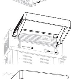
$\underline{\texttt{STEP 24}}$  Use two (2) M5x10 screws to attach the power cord bracket to the back of the air fryer.
