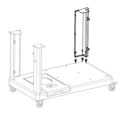
**STEP 05** Use two (2) M6x15 screws (**a**) to attach the front-right leg to the cart base.
