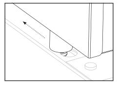
Ensure that the front pins are seated in the holes, then push the griddle top back to lock the griddle in place. **STEP 32** Open the hood. **With the help of another person**, place the griddle top on the main body by aligning the four (4) pins to the holes of the body. Make sure the front pins are fully seated in the holes, then push the griddle top back to lock the griddle in place.
