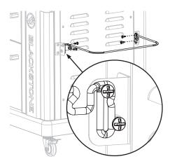
**STEP 26** Use eight (8) M6x15 screws (**a**) to install the four (4) side shelf brackets. (One side shelf bracket **A** and one side shelf bracket **B** per side.)
