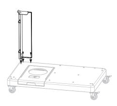
**STEP 03** Use three (3) M6x15 screws (**a**) to attach the front-left leg to the cart base.
