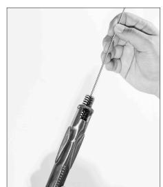
**STEP 04** Brush entire outer surface of burner to remove grime.
