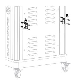
**STEP 25** Use four (4) M5 step bolts (**d**) to attach the garbage bag holder to the garbage bag holder brackets.
