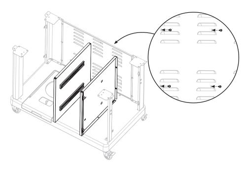
**STEP 08** Use three (3) M6x15 screws (a) to attach the left drawer panel to the cart base.
