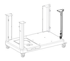
**STEP 06** Use six (6) M5x10 screws (**b**) to attach the back panel to the rearleft leg and rear-right leg.
