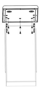
**STEP 19** Insert one (1) drawer handle into two (2) handle standoffs. Use two (2) M6x15 screws (**a**) to attach one (1) drawer handle to the lower drawer front panel.
