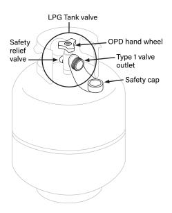
Always keep new and exchanged LPG Tanks in upright position during use, transit or storage.
