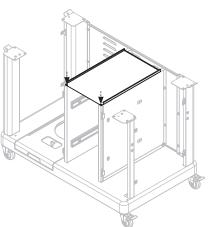
**STEP 11** Use four (4) M5x10 screws (**b**) to attach the top bracket to the front-left and front-right legs, and secure the drawer heat shield to the left and right drawer panels.
