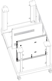
**STEP 10** Align the holes on the drawer heat shield with the holes on the left and right drawer panels.
