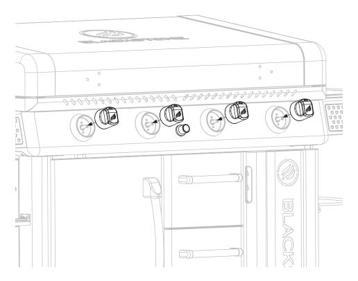
**STEP 31** Insert the hood handle into the two (2) handle standoffs. Use six (6) large M6 step bolts (**f**) to attach the handle to the griddle hood.
