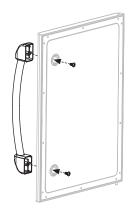
**STEP 16** Attach the left cart door to the cart by first **1** inserting the door into the upper door hinge pin, then **2** inserting the lower door hinge pin into the cart base.
