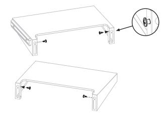
**STEP 14** Hook the left side shelf's M6 step bolts onto the shelf brackets on the left side of the griddle.
