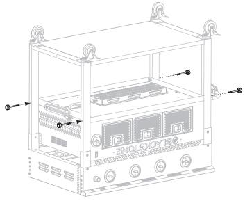
**STEP 04** Slide the legs into the slots on the griddle body and use two (2) M6x12 screws on each of the four corners to secure them to the griddle body.
