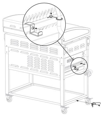
**STEP 11** Use two (2) M6x12 screws to attach the power cord bracket to the right leg assembly.
