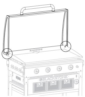
Place one (1) hood spacer between the hood and the griddle top, the small end into the hood and the large end into the griddle top.
