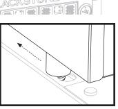
STEP 08 Use two (2) M6x12 screws and two (2) hood handle bezels to
