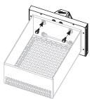
**STEP 15** Hang the grease cup in the slot on the back of the griddle body.
