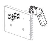
Re-attach the front panel with the previously removed thumb screws. Repeat this step with the other two (2) drawers.
