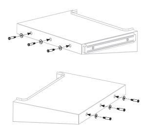
**STEP 13** Thread two (2) M6 step bolts into the top holes on the left side shelf and two (2) M6 step bolts into the top holes on the right shelf.
