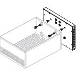
**2** Use four (4) silver countersunk M5x15 screws to attach the drawer handle to the front panel. Be sure to install handle correctly, with the handle facing down.
