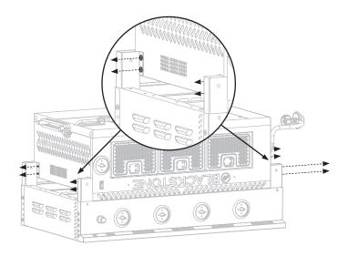
**STEP 05** Use four (4) M6 thumb screws to secure the legs to the airfryer body.
