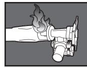
POSSIBLE CAUSES Something is blocking the venturi in the burner tube. **SOLUTION** Clean the burner assembly to remove the obstruction.
