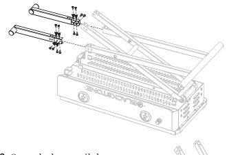
**STEP 06** Open the legs until the top of the wheeled leg assembly aligns with the C clamps.
