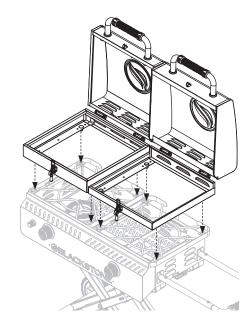
**STEP 16** Use eight (8) clips to secure the grill box and the griddle box to the tailgater.
