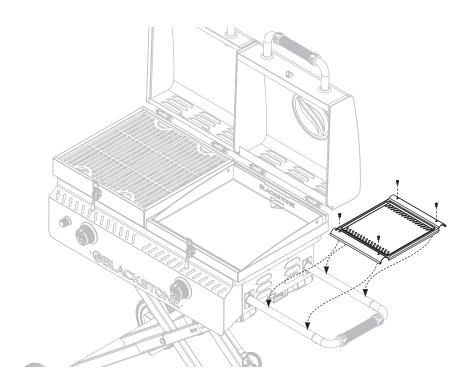
**STEP 19** Use four (4) hexagon bolts to attach the side shelf to the left side off the griddle body.
