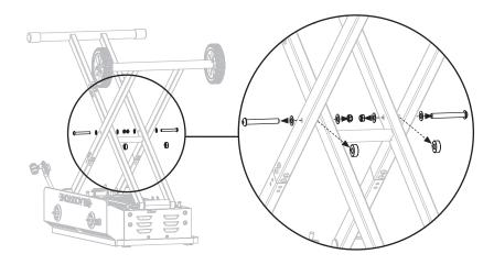
**STEP 10** Use the two (2) removed bolts, four (4) removed washers, two (2) removed nuts and two (2) removed spacers to attach the lower bracket to the leg assemblies.
