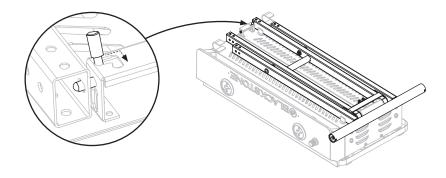
**STEP 05** Raise the legs, and use twelve (12) M6x12 bolts to install the upper legs onto the wheeled leg assembly.
