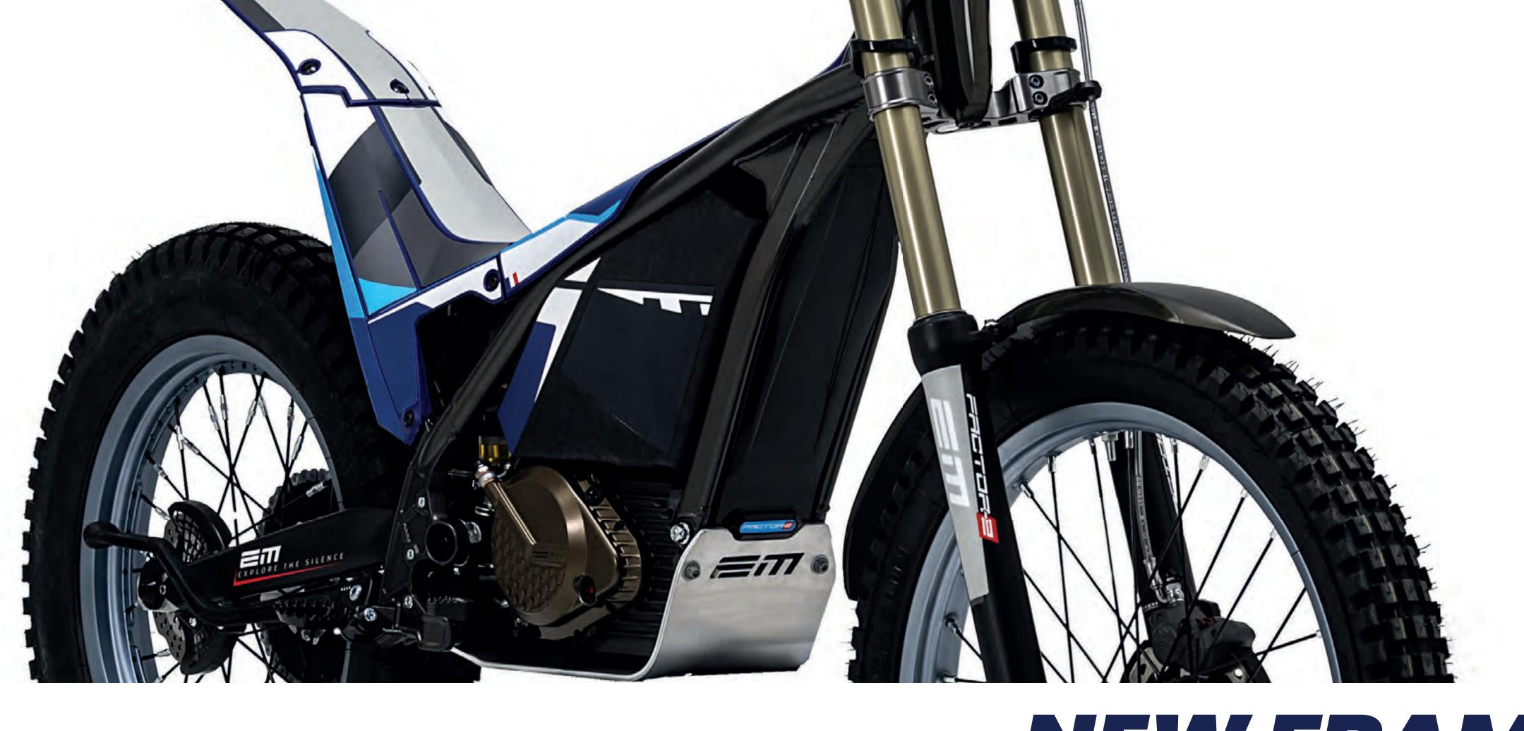
The steering-column assembly has been redesigned and stiffened to further enhance steering precision and the triple clamps have new offsets for a more dynamic front end.
