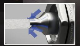
With Split Nozzle<sup>™</sup> 2.0 air is forced into the centre of the paint jet stream, this pre-atomises the material before it reaches the air caps.
