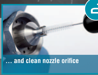
2 Clean the material with a brush (art. nr. W2COM6126 )
