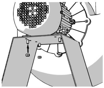
5. Ensure that the motor is completely secured to the support stand before running the blower.
