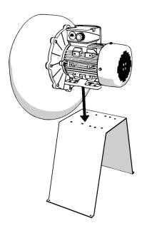
3. Insert the 4 supplied bolts through the feet of the motor and the top of the motor support stand.
