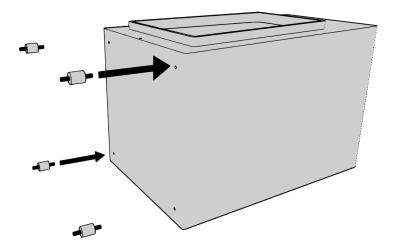
4. Through the opening in the rear, secure the vibration isolators to the weather hood with the provided nuts.
