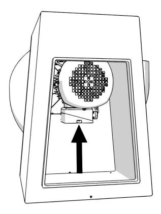
4. Insert the provided bolts through the feet of the motor and through the top of the weather hood.
