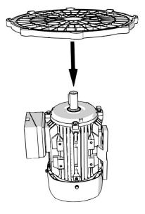
3. Secure the motor plate screwing the 4 bolts and washers through the plate into the C face of the motor.
