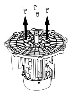
8. Remove the motor plate from the C face of the motor.
