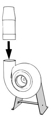
3. Secure the speed nozzle to the blower outlet. Drill four evenly spaced holes through the speed nozzle and into the blower outlet. Insert screws into the holes to secure the speed nozzle.
