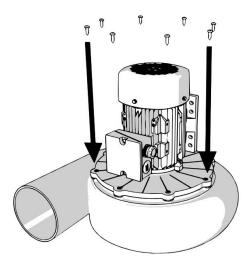
10. Orient the fan so that the inlet is accessible. Ensure that the impeller can rotate freely and does not rub on the blower housing.
