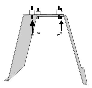
4. Place the blower assembly onto the vibration isolators.
