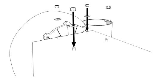
6. Ensure that the blower is completely secured to the weather hood before running the blower.
