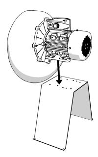
3. Insert the 4 supplied bolts through the feet of the motor and the top of the motor support stand.
