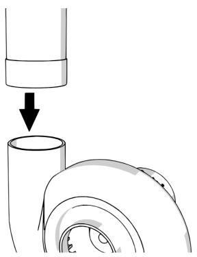
3. Secure the stack to the blower outlet. Drill four evenly spaced holes through the stack and into the blower outlet. Insert screws into the holes to secure the stack.
