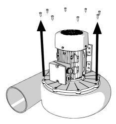
3. Pull the motor assembly from the blower housing. It may require some force to unseal the motor plate from the blower housing. Be careful not to damage the impeller.
