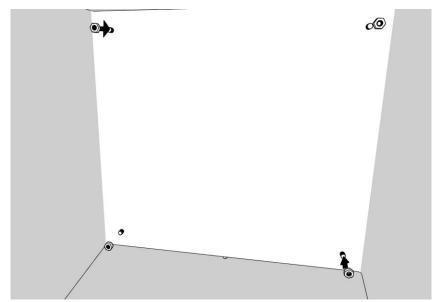
5. Ensure that the vibration isolators are properly secured to the weather hood before installing the blower.
