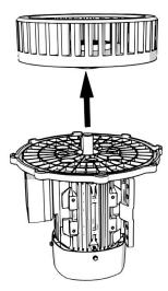
7. Remove the 4 bolts going through the motor plate into the C face of the motor.
