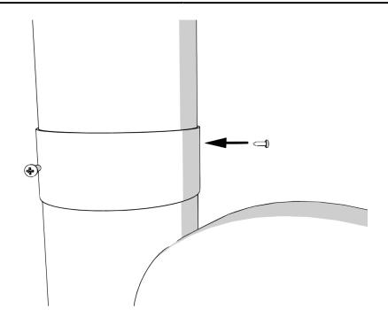
4. Ensure that the stack is properly secured before starting the blower.
