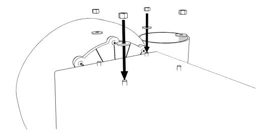
6. Ensure that the blower is completely secured to the weather hood before running the blower.
