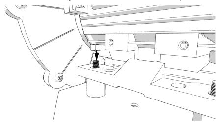
6. Ensure that the blower assembly is properly secured to the motor stand and vibration isolators before running.
