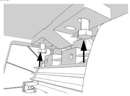
5. Place the provided washers over the bolts that are protruding through the top of the weather hood. Secure the bolts and washers with the provided nuts.
