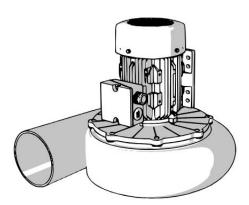
2. Remove the T25 Torx head screws from the motor plate. (There will be 8 or 16 screws depending on the blower. There may be a screw already missing in front of the motor junction box)
