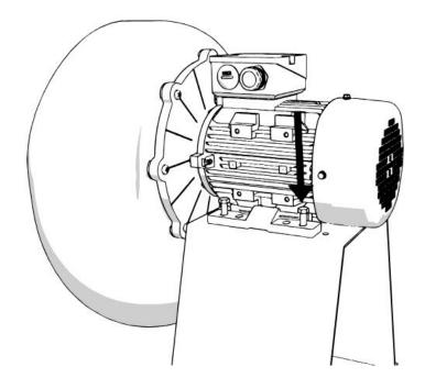
4. On the underside of the motor support stand, thread the 4 supplied nuts onto the bolts. Tighten the bolts and nuts to fully secure the blower to the motor support stand.
