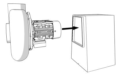
3. Hold the blower against the roof of the weather hood and align the holes in the feet of the motor with the holes drilled into the top of the weather hood.
