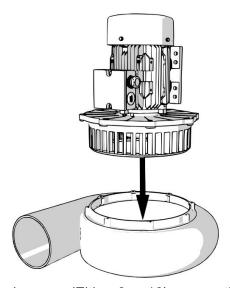
9. Using the supplied Torx head screws (Either 8 or 16), secure the motor assembly to the blower assembly. Depending on the supplied motor, one screw may not be able to be screwed in due to the size and placement of the motor junction box.
