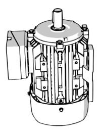
2. Set the motor plate onto the C face of the motor. It may require a small hammer or dead blow mallet to set the plate onto the rabbet. It will not require that much force to properly seat the motor plate.
