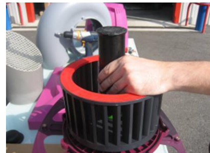
6. Push in the impeller.
