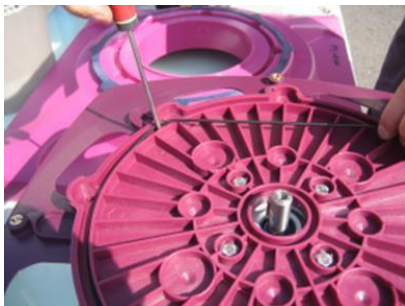
4. Place the O-ring seal.
