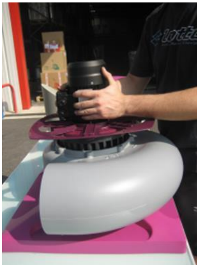
13. Place the motor/impeller part.
