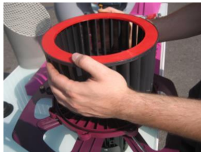
5. Place the impeller.
