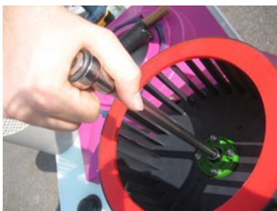
7. Screw the hub cap on the motor shaft.
