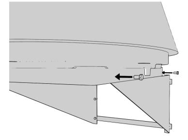
5. Secure the bolts with corresponding nuts.
