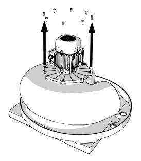
7. Pull the motor assembly from the blower housing. It may require some force to unseal the motor plate from the blower housing. Be careful not to damage the impeller.
