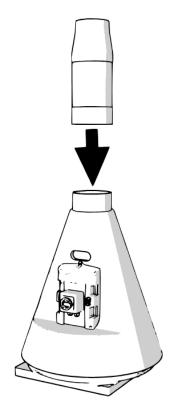
3. Secure the speed nozzle to the blower outlet. Drill four evenly spaced holes through the speed nozzle and into the blower outlet. Insert screws into the holes to secure the speed nozzle.
