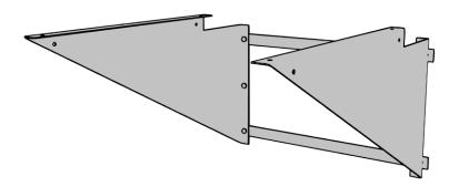
2. Place the JET on the Wall Bracket. Ensure that the wall bracket is seated properly within the roof cap base of the JET.
