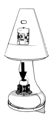
8. Ensure that the blower is properly secured before running.
