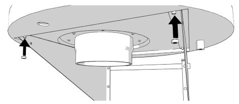
7. Reinstall the JET Cone. See 7.3.2 Assembly/Reassembly Instructions for reinstalling the cone.
