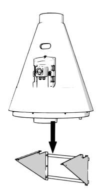
3. Remove the cone of the JET. See *7.3.1 Disassembly Instructions* for removing the cone.
