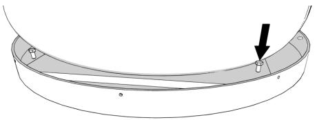
6. Secure the bolts with corresponding nuts.
