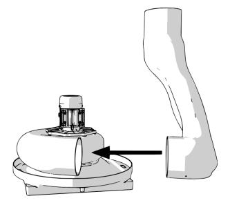
10. Slide the cone over the exhaust manifold and onto the base of the JET. Ensure that any wiring does not interfere with the JET cone.
