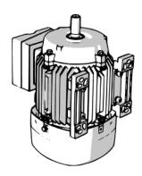
2. Set the motor plate onto the C face of the motor. It may require a small hammer or dead blow mallet to set the plate onto the rabbet. It will not require that much force to properly seat the motor plate.
