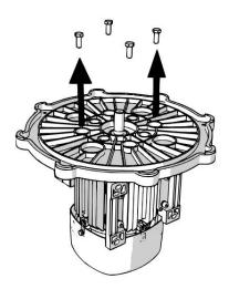
12. Remove the motor plate from the C face of the motor.
