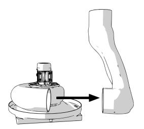
6. Remove the T25 Torx head screws from the motor plate. (There will be 8 or 16 screws depending on the blower. There may be a screw already missing in front of the motor junction box)
