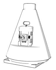
2. Open the disconnect switch on the front of the JET cone. Remove the wiring from the disconnect switch and feed through the hole in the back of the switch housing. Take note of the order of the wiring before removing it.
