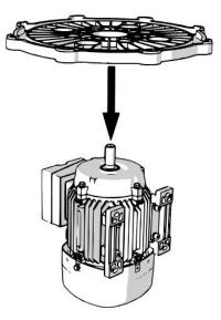
3. Secure the motor plate screwing the 4 bolts and washers through the plate into the C face of the motor.
