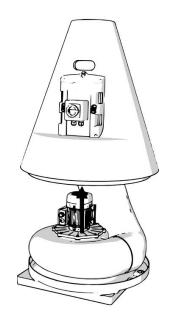
5. Remove the exhaust manifold from the outlet of the blower housing.
