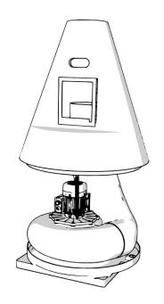
11. Feed the wiring through the rear of the JET door and into the disconnect switch.
