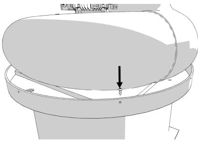
7. Reinstall the JET Cone. See 7.3.2 Assembly/Reassembly Instructions for reinstalling the cone.
