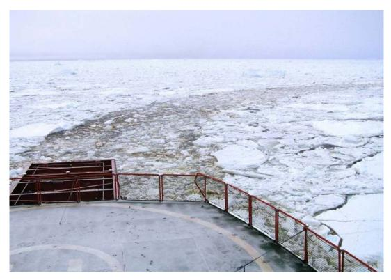
There is a big fence around the edge of the helideck that folds outwards during heli-operations and it had to be put upright again for the voyage, and some of us helped with that, pulling the panels up with a rope, then slipping bolts into the hinges to keep them there. It was a simple job made difficult by the cold and made me appreciate the work the crew were doing.
