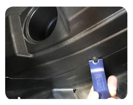
**Step 6** - Routing Main Harness. Now that the center console is out of the way, take the main wire harness and place it through the fire wall (amplifier connectors side).
