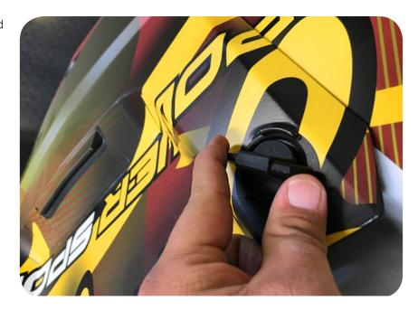
**Step 2** - Remove Top Dash Panel. Using your Torx screwdriver, unbolt the two factory bolts. Using your hands, pull the top dash piece toward the interior of the vehicle to release it from the dash. Disconnect all of the wires connectors and set aside.
