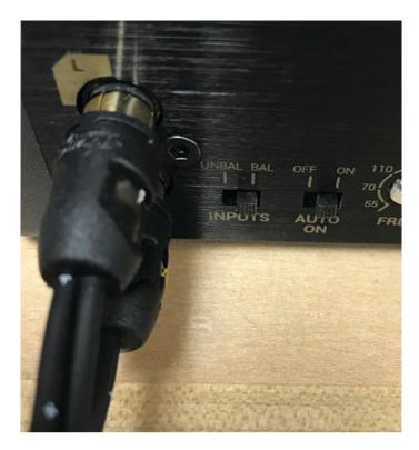
On PG SX2 and Ti3 Amplifiers - When the amplifier is in the OFF mode - Move the inputs switch to BAL and plug your RCA's in naturally
