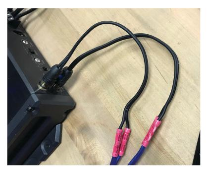
Simply strip the end of the Z12LINE and connect the + & - according to the printed cable housing to the + & - on your standard Stinger speaker wire.
