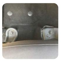
3. Place the seat in the full rearward position and remove the two 18mm front seat bolts.
