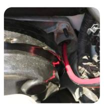
5. Cut or poke a hole in the membrane. Run the power wire through the membrane into the vehicle.
