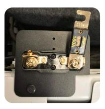
5. Align the mounting holes to the plate and install two of the supplied screws.
