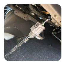
5. Tilt the seat up and disconnect the electrical connector.
