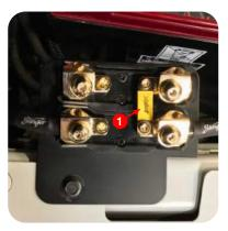
1. To connect the two X-Links, align the locking channels on the bases and press together. Install the two mounting screws. You can run a new power wire to the second X-Link, or you can use the X-Pansion Jumper (1) to pass power from the first X-Link to the second.
