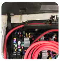
5. Starting at the fuse holder, route the power wire inside the wire cover.
