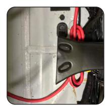
2. If the power wire is too long, it can be cut to length and a new ferulle installed (see below). If the power wire is just a bit too long, there is plenty of room under the carpet to store some slack and leave the factory installed ferrule attached.
