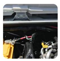
2. Running the wire on the top of the harness provides the most protection and least visibilty.
