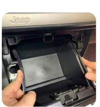
4. Remove the glove box by pushing inward on both sides and lowering to unhinge the bottom.
