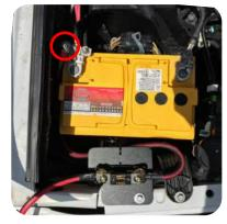
2. Remove the 10mm bolt on the positive battery terminal. Install the eyelet on the terminal stud. Reinstall the 10mm nut and tighten securely.
