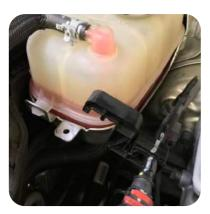
2. Unclip the hose attached to the coolant reservoir.
