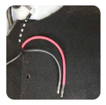
8. Route the ground wire under the carpet and out the opening in the carpet.
