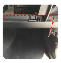
5. Route the power wire across the glove box opening following the factory wire harness. Secure with zip ties.
