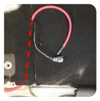
6B. DRIVER SIDE: Route the power wire down from the upper dash area where it enters the vehicle, to the kick panel harnesses, then along the door jamb, and finally out under the seat through the opening in the carpet.
