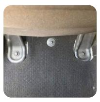
4. Move the seat to the forward position and remove the two 18mm rear seat bolts.
