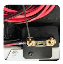
7. Insert the braided sleeved end of the XX power cable into the left side of the fuse holder and tighten the 4mm set screw.
