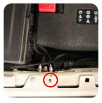
1. The fuse mounting plate will be attached to the passenger side fender near the battery using the threaded hole indicated.
