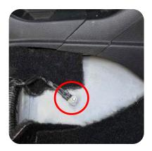
7. On both sides of the center console there will be a factory ground point. Remove the 10mm nut and attached the Black 12in Ground lead. Retighten the nut securely.
