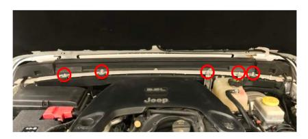
1. Remove the five 10mm nuts securing the plastic wire cover and coolant reservoir.
