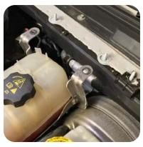
3. Lift the reservoir off the studs and position out of the way.
