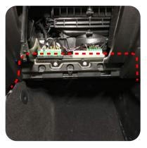
6. Route the power across the glove box opening following the factory wire harness running behind the green and white distribution blocks. Secure with zip ties.
