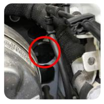
7. Remove the plastic insert located to the right of the brake booster.
