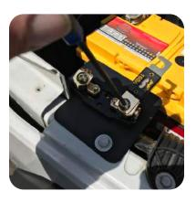
4. Temporarily loosen the 4mm fuse set screws and move the fuse to access the two mounting holes in the base.
