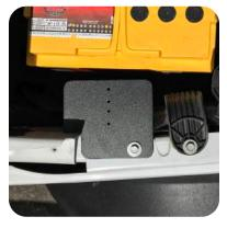
2. Remove the 10mm bolt and attach the fuse mounting plate in the direction shown above.
