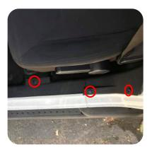
1. Remove the three push fasteners on the door sill panel and lower B pillar trim.
