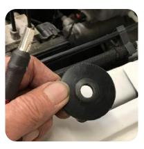
8. Drill a 5/8" hole in the plastic and install the supplied rubber grommet.
