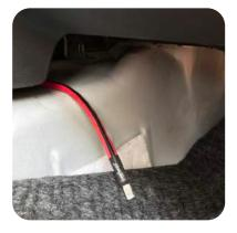
3. Pull back the carpet on the passenger side of the center console and pull the lenght of wire through to the passenger side.
