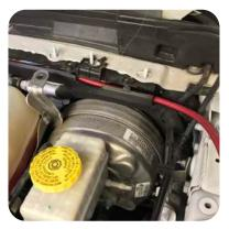
6. Continue routing the power wire inside the plastic cover to the driver's side of the vehicle.
