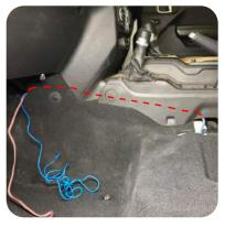
4. Route the cables forward, tucking them behind the center console side panel and carpet. NOTE: Complete Step 1 on the next page before routing the wires any further.
