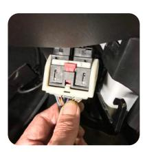
3. Disengage the red lock and disconnect the connector.
