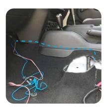
10. Route the cables forward, tucking them behind the center console side panel and carpet. NOTE: Complete Step 1 on the next page before routing the wires any further.
