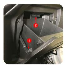
5. Remove the glove box by detaching the arm on the left side (1), and then pushing up on the stop at the top (2). Lower fully to unhinge at the bottom.
