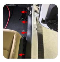
4. Remove the kick/door jamb panel by pulling it towards the center of the vehicle.
