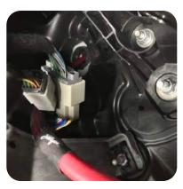
1. Inside the vehicle, secure the power wire to the factory wire harness on the left side. If mounting the amplifier under the drivers seat, skip to Page 13.
