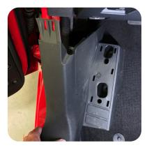
6. Pull the kick panel towards the rear of the vehicle to release the remaining locking clips.
