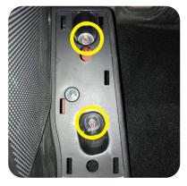
2. Driver's Side Only: Remove the two 10mm nuts securing the foot rest to the floor.
