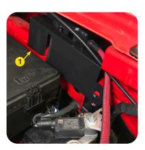
3. Position the mouting plate under the fender and slide the tongue down into the pocket (1).
