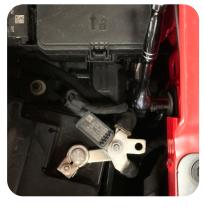
2. Remove the 13mm bolt and set aside.
