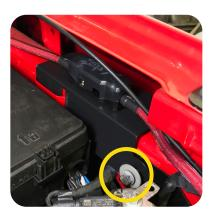
4. Align the bolt hole on the mounting plate and reinstall the 13mm bolt.
