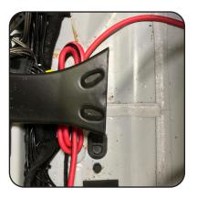
6. If the power wire is too long, it can be cut to length and a new ferulle installed (see below). If the power wire is just a bit too long, there is plenty of room under the carpet to store some slack and leave the factory installed ferrule attached.
