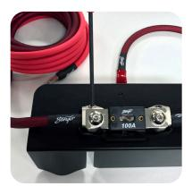
7. Insert the braided sleeved end of the 17' power cable into the left side of the fuse holder and tighten the 4mm set screw.
