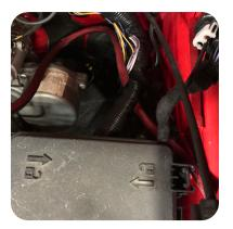
2. Route the long end of the power wire to the grommet. Lubricate the wire and pass it through the grommet into the inside of the vehicle.
