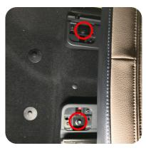
11. Position the front seat fully rearward. Remove the two front seat bolt covers (1). Remove the two 13mm seat bolts. Position the seat in the full forward position.
