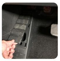
1. Driver's Side Only: Using a panel tool, remove the tread plate from the foot rest.
