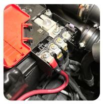
2. Install the ring termininal on one of the empty studs on the positve battery terminal. Secure with the M6 flange nut included in the kit.
