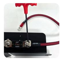
6. Loosen the wire set screw on the right side and insert the 22" power lead and tighten securley.
