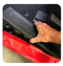
3. Remove the front door scuff plate by pulling upwards to release the retaining clips.
