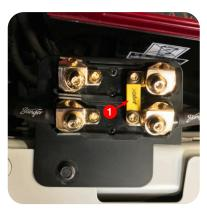
1. To connect the two X-Links, align the locking channels on the bases and press together. Install the two mounting screws. You can run a new power wire to the second X-Link, or you can use the X-Pansion Jumper (1) to pass power from the first X-Link to the second.
