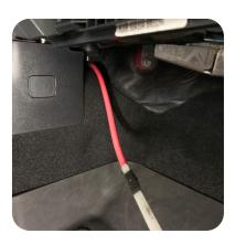
4. Feed the power wire from the driver's side to the passenger side in front of the center console.
