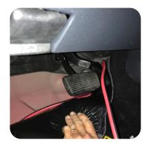
3. Route the power wire from the driver's kick panel to the front of the center console under the carpet.
