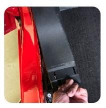
4. Release the clips securing the back end of the kick panel by lifting upwards.
