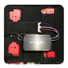
5. At this point, the amplifier should be set in place. If using an amp mounting bracket, the amplifier should be attached to the bracket and then set in place. For each connection, ensure there is the proper amount of wire lenght..
