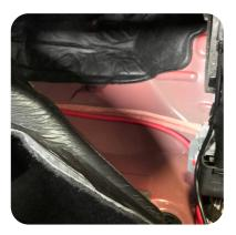
5. Pull back the carpet on the passenger side. Route the power wire to the passenger kick panel.
