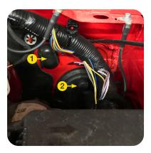
1. If there are two rubber grommets available behind the fuse box, use #1. Using a utility knife or diagonal cutters, cut a slit in the grommet.
