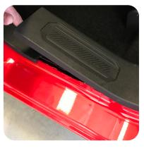
8. Remove the rear door scuff plate by pulling upwards to release the retaining clips.
