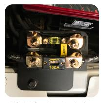
2. X-Link inputs and outputs can accept 0/1, 4 and 8 GA wire. ANL or MIDI fuses can be used, or a combination of both as shown above.
