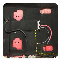
2. Route the ground wire under the carpet from the B pillar to the opening under the seat.
