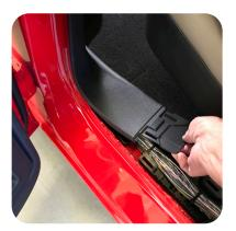
9. Pull up and release the clips on the lower B pillar trim inside the rear door.
