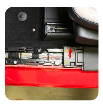
7. Pull up and release the clips on the lower B pillar trim inside the front door.
