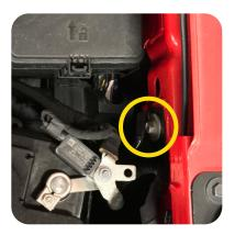
1. In the engine compartment, on the driver's side, locate the 13mm bolt on the inner fender between the battery and the fuse box.
