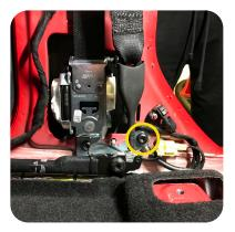
1. At the base of the B pillar, attach the black ground wire using the bolt indicated. Tighten securely.
