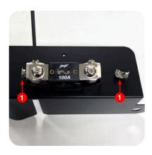
5. If installing the 4GA kit, remove the 8GA inserts (1) from both ends of the fuse holder by losening the 4mm wire set screws.
