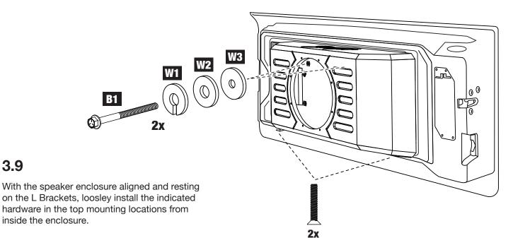
Install the two 4mm allen hex screws removed in Step 3.1 into the bottom locations.
