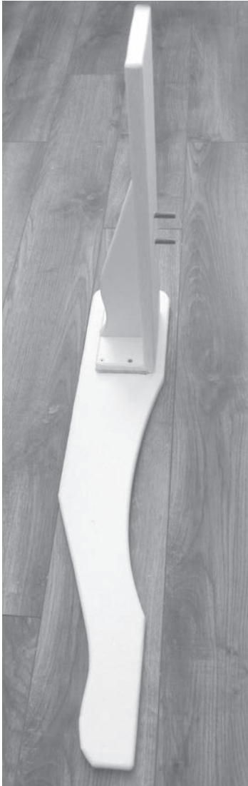
Finished Left Arm Assembly
