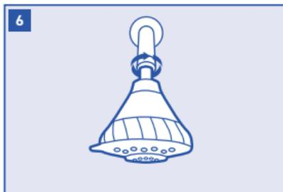
Place showerhead on piping and tighten by hand turning clockwise.
