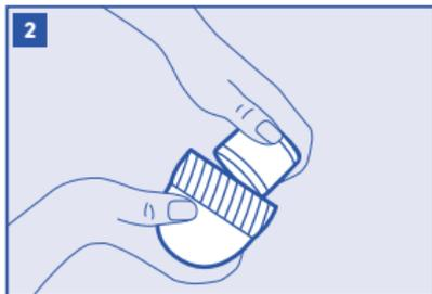
Grasp white filter cartridge and pull cartridge up and to the side to remove and discard.
