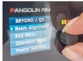
C: Find Beam Alignment option in the menu and enter it by pressing the rotary knob.
