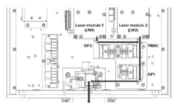
8. Create a full size red circle (static tunnel effect) and check whether the red circles of all R4, R3, R2 and R1 overlay each other all the way around the shape. If not, follow the diagram below to adjust the beam path accordingly (step 1 on the diagram below).
