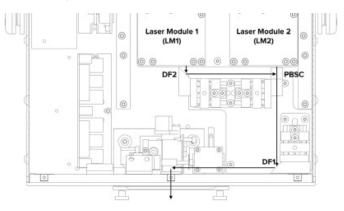
Create a full size red circle (static tunnel effect) and check whether the red circles of all R4, R3, R2 and R1 overlay each other all the way around the shape. If not, follow the diagram below to adjust the beam path accordingly (step 1 on the diagram below).
