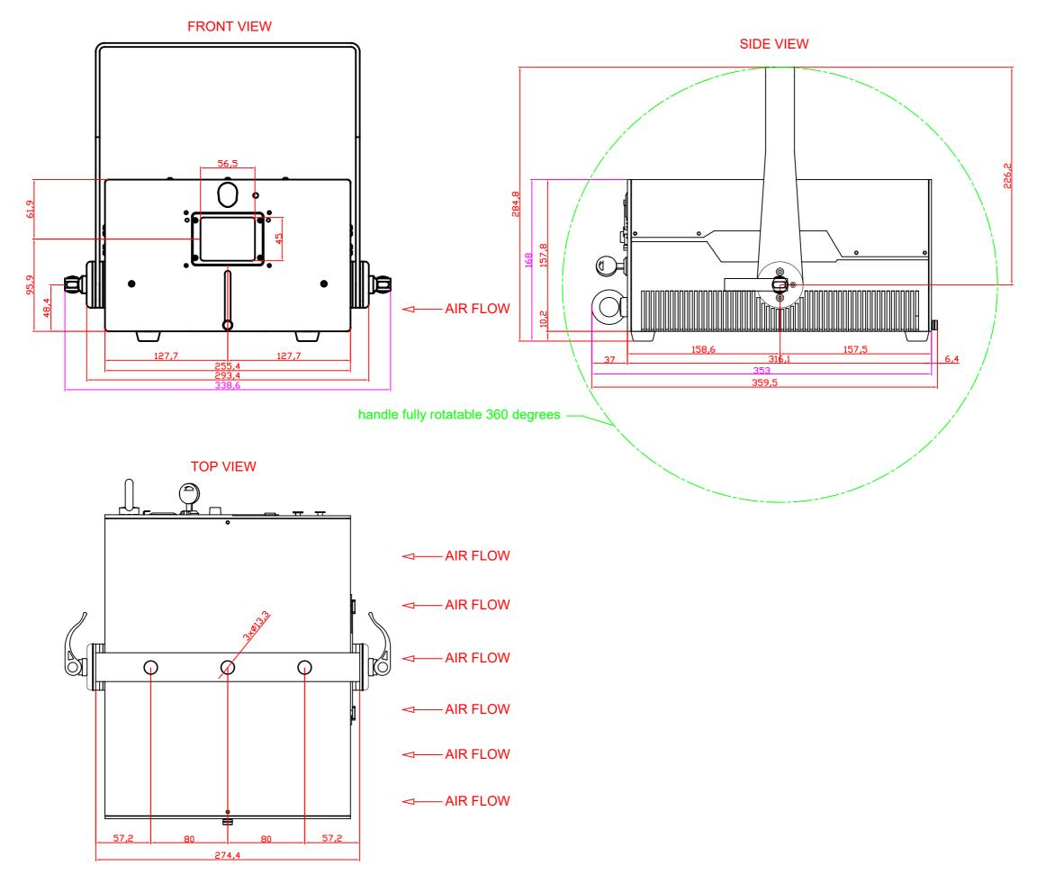
Purple: Overall dimensions, including all the fittings and extrusions; without the 360° swivel bracket Total airflow needed for the laser projector: 60 cubic metres per hour
