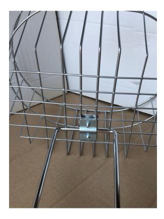
Next, loosen the handle bar stem, head sets (lock nut and spacer) from the bike, loop the basket bracket onto the headset area (to replace the spacer you took out earlier). Screw the headset (locknut) back, install the stem back to the bike.
