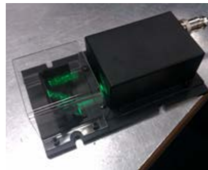
Light source with beam detection designed for laser labyrinth
