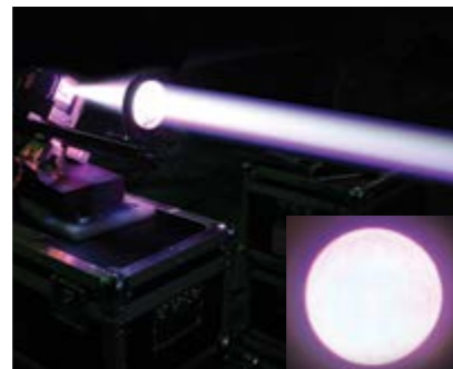
Round low divergence laser beam with homogeneous intensity distribution
