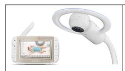
The EUTs are Over-the -cot Wi-Fi® Monitor and sleep companion system which consist of a baby unit and a parent unit, the baby unit supports Wi-Fi 802.11 b/g/n and general 2.4GHz wireless technologies, and the parent unit only supports general 2.4GHz wireless technology.
