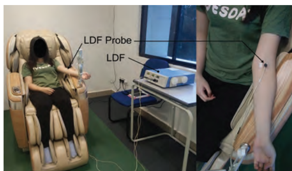
Fig. 3. A laser doppler flowmeter (LDF) is used to measure the SBF by positioning the LDF meter probe on the antecubital fossa region.
