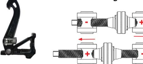
Floated and Fixed bearing balance bars adjust in opposite directions but the most pedal force will always go to the the master cylinder that is the closest to the bearing.
