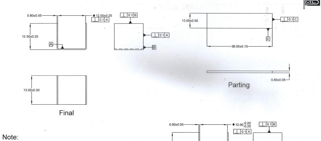
Unless otherwise specified, tolerance as per ISO 2768-class m
