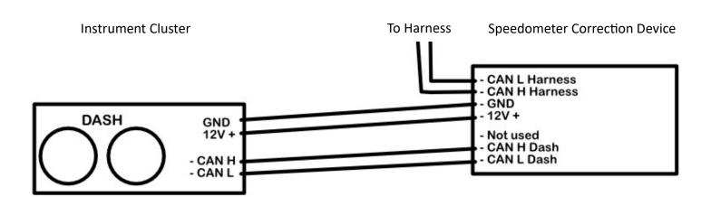
Once all has been connected as required carefully cable tie the speedometer correction device somewhere in the dash so that it is out of the way and securely fastened. Run the unit so it can be accessed while test driving.
