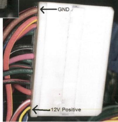
**Note:** The **grey & blue** and **white & brown** wires must be twisted together before they are joined to the original vehicles wiring harness.
