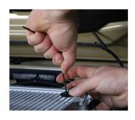
Push the locking button onto the quick mount rod to sit flush with the face of the intercooler. Cut off excess quick mount rod.
