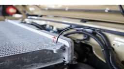
With a screwdriver carefully notch out a small hole within the radiator fins to feed the quick mount rod through. (AS SHOWN ABOVE)
