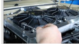
Peeling off the protective plastic wrap before tightening bolts is advised.
