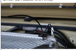
Feed temperature probe and quick mount rod through locking button. Insert the temperatire probe between the seperated fins.
