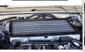
Remove the nuts and bolts from the standard intercooler and place aside. After removing the bolts remove the black plastic cover from above of the intercooler. (AS SHOWN BELOW)
