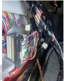
Cut and solder the yellow paddle shift receiver cable to the ignition wire
