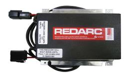
The voltage regulator operates in a 24 V DC automotive electrical system providing a safe 12 V output for 12 V equipment. It is a low noise voltage regulator designed for use with sensitive radio communications equipment. The maximum output is 20 Amps. The conversion efficiency at full load is more than 90%.
