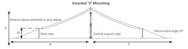
Note: Antenna should be orientated at broadside to the preferred direction of communication to maximise signal level. Horizontal configuration should be used for medium to long distance communications, and inverted-V for short to medium distance.
