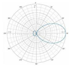
If the antennas are mounted for vertical polarization, these curves show the radiation patterns in the vertical plane.
