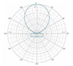
If the antennas are mounted for vertical polarization, these curves show the radiation patterns in the horizontal plane (horizontal coverage).
