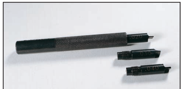
This handy tool is an inexpensive way to nick flat or rotary dies. Comes complete with 3 tip sizes - .020", .030" & .040". Special tips are available. .010", .015", .050", .060", .070" and .080". Tips up to .030" should only be used on medium hard rule or softer.
