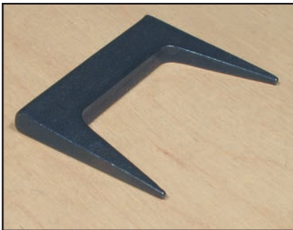
Used to hold dieboards tight while inserting corrugated fasteners. Can also be used to secure rotary dieboards together when being bolted to drum. 2" long x 1-1/2" high.
