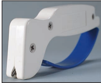
CCM Die Supply stocks three different models, (left to right) the "Super Sharpener", the Economy style and the Sharpy Rule Sharpener. Recommended for use on dies which cut into a cutting pad. Should be used only to touch-up rule to help complete a cutting job.
