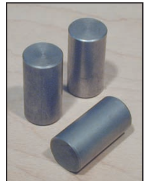
Precision ground, solid steel stop pins help protect steel rule die from damage as a result of uneven press conditions.
