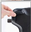
Remove the rear factory feet by removing the two screws holding them in place, taking note of the screw sizes and the holes from which they were removed.
