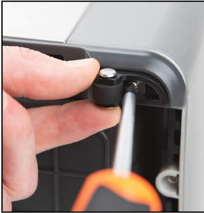
Pair a triangular washer with a front foot housing by sliding the washer onto the screw and then inserting the screw into the housing.
