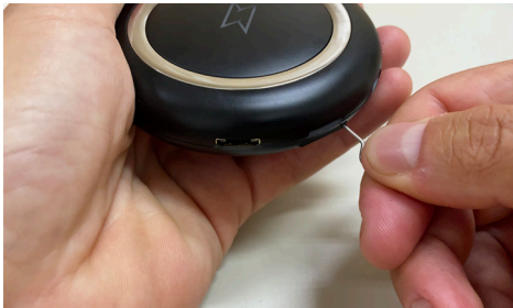
2 - Use the removal clip to eject and remove the SIM card compartment.
