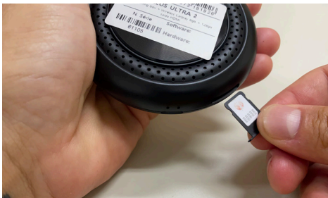
3 - Turn the device upside down, place the SIM card in the compartment as shown in the photo above and insert it into the SIM card slot on the ZEUS ULTRA 2
