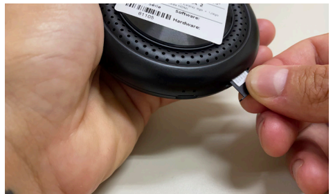
3 - Turn the device upside down, place the SIM card in the compartment as shown in the photo above and insert it into the SIM card slot on the ZEUS ULTRA 2
