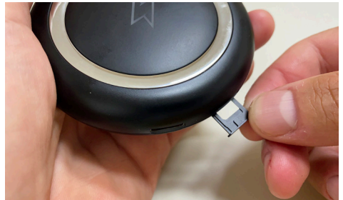
2 - Use the removal clip to eject and remove the SIM card compartment.
