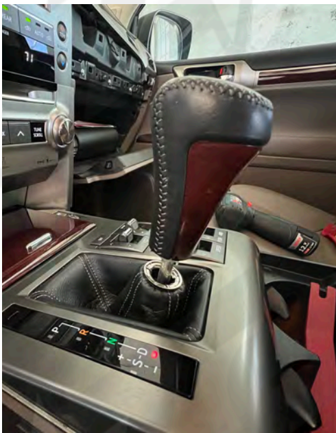
4. Pull down the shifter shroud (clipped in only)
