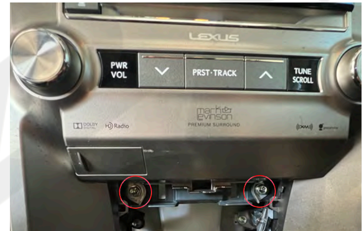
8. Remove trim panel, and remove (2x) 10mm bolts hidden behind it.
