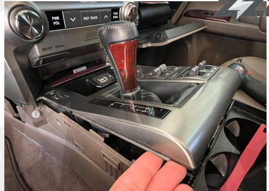
6. pull up this dash piece after removing the shifter.
