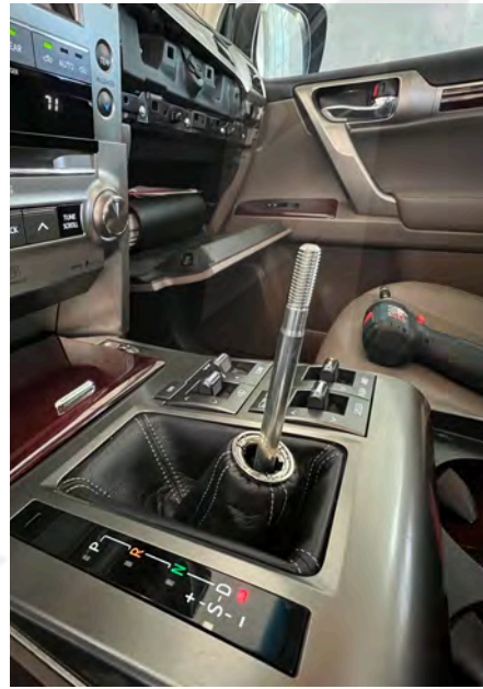
5. Remove the shifter by twisting it off.
