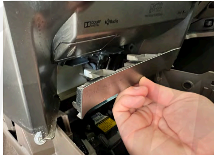
8. Remove trim panel, and remove (2x) 10mm bolts hidden behind it.
